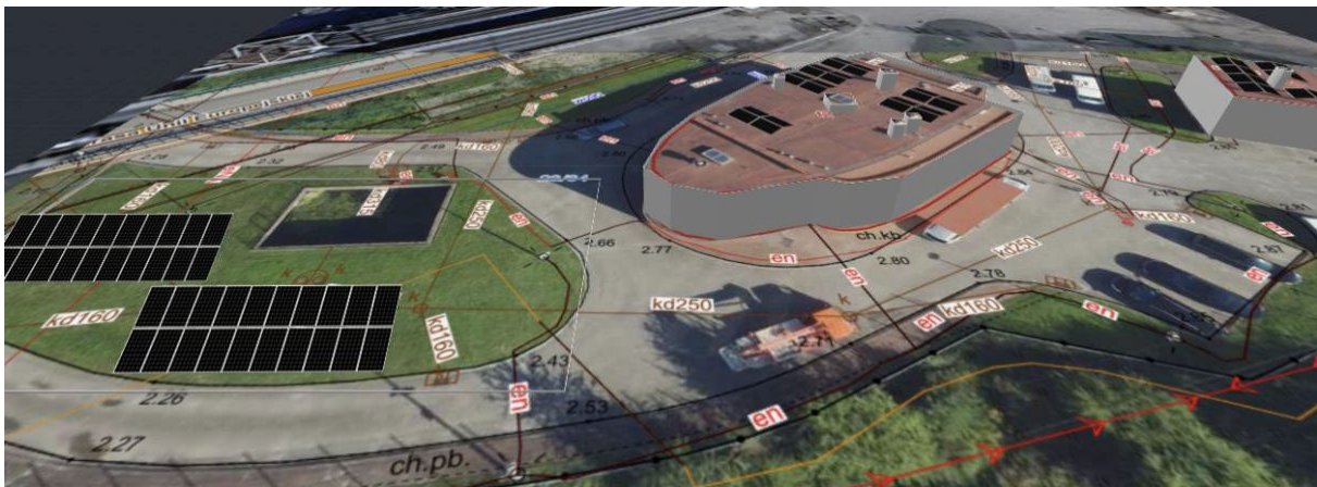
Figure 57. Visual presentation of the solar panels' placement in the Port of Elbląg Source: Voltaic System
